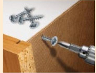
**The flat surface under the head does not generate the undesired "wedge effect"** caused by flat countersunk head screws. The wide area under the head also provides **high back panel pull-out strength**.
