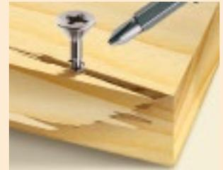
*Screwing with traditional chipboard screw without pre-boring.*
