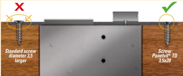
The **reduced head (Ø 6 mm)** allows to use a diameter screws (3,5) that **guarantees better tightness**, without that the head come out from the hardware.
