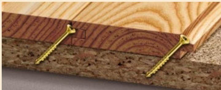
**The reduced head with milling ribs and TX hexalobular recess** bites into the wood without causing splitting while tightening. **Head completely penetrates into the wood to allow the interlocking of the next strip.** The TX recess transmits all the screwing force and prevents slipping and wear in the recess.
